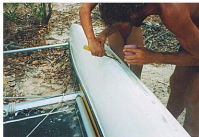
**And this is the result. We had to take the mast down and turn the boat upside down, then start filling the gaps with repair resin. I'm holding the gap open while Dad stuffs the goop inside.**
